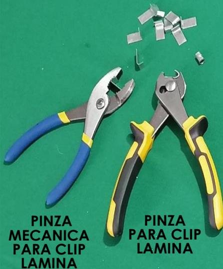
PINZA MECANICA PARA CLIP LAMINA
