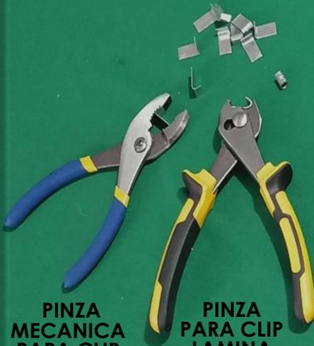
PINZA MECANICA PARA CLIP LAMINA
